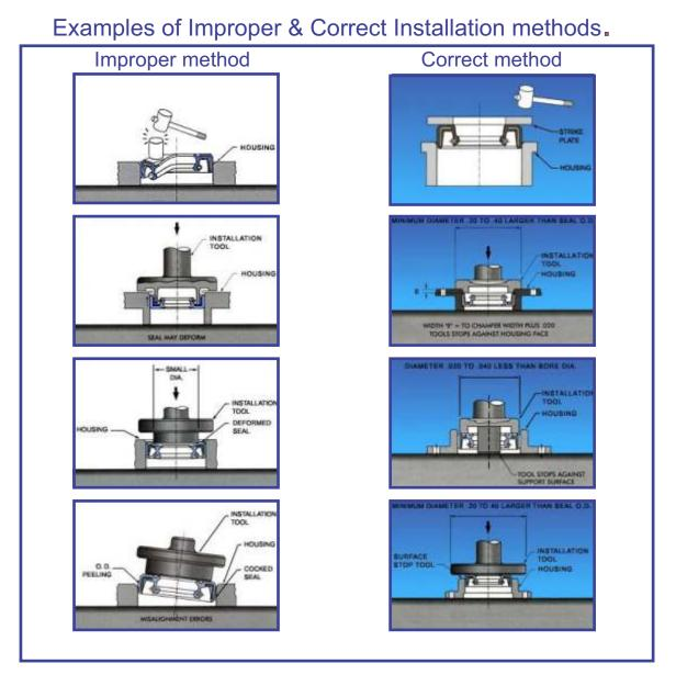
Proper tools and method are required for of good installation of seal, with the right amount of force, if seal is not installed properly than it could damage the other parts of the assembly, it could lead to unplanned and unwanted friction, heat, and wear, all of which can contribute to premature seal failure.
